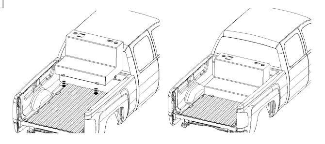
Using a marker, mark the hole location in the four tank attachment points.
