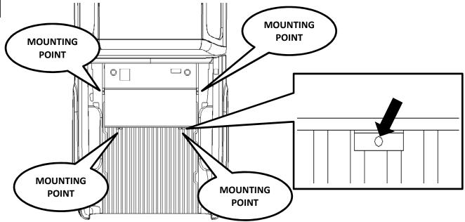
Check the underside of the truck bed below the marked locations for clearance. If something is in the way of the marked location, shift the tank to avoid the obstruction.
