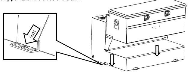
At the side mounting locations, place a 5/16" bolt [B] and 5/16" washer [C] down through the mounting location hole. From the underside of the truck place a rubber bumper [E], 5/16" washer [C], and 5/16" lock nut [D] onto the bolt.
